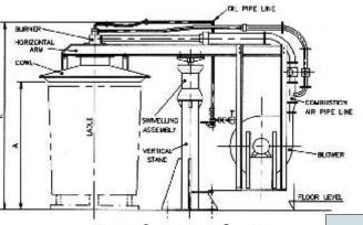
The ladle preheater is fitted with a Wesman oil burner with Sensitrol oil valve (LPG or natural gas firing is also available as an option) to obtain a maximum drying temperature of 1000°C. Combustion air is provided by Wesman centrifugal blower. Preheated oil at constant temperature and pressure is supplied to the burner by a Wesman oil heating and pumping unit.
